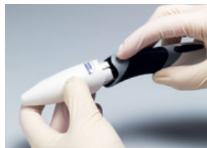
Fig.: Batteries should be easy and quick to remove.
