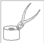
After casting allow the moulds to cool down until warm to the touch, **do not quench in water!** Investment materials contains quartz. Do not inhale dust! Danger of lung harms (silicosis, lung cancer). To avoid dust during deflasking, place the moulds in water after they have cooled down completely after casting until they are thoroughly moistened.
