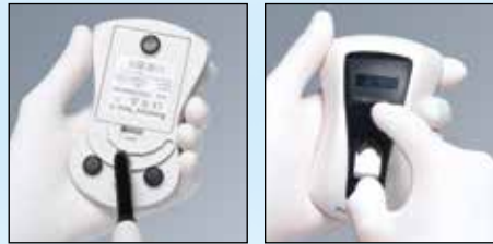
The diameter of circular light guides is measured by means of the gauge on the back of the radiometer.
