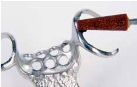
Finishing with corundum or fine grinding stones
