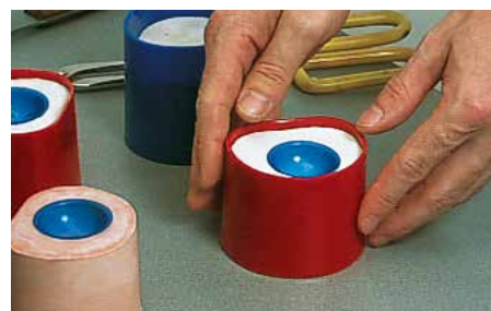
Hardening time 30 minutes for the conventional casting
