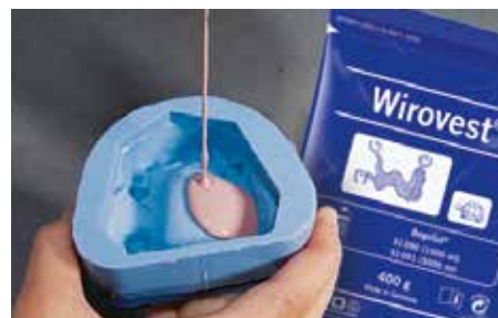
Filling of partial denture investment material
