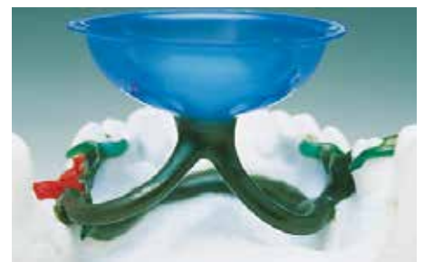
Sprue attachments in lower jaw, casting from above
