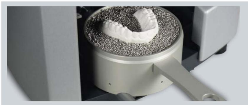
It is possible to thermoform on a model plate or in granules. The handling of the granules was significantly improved.
