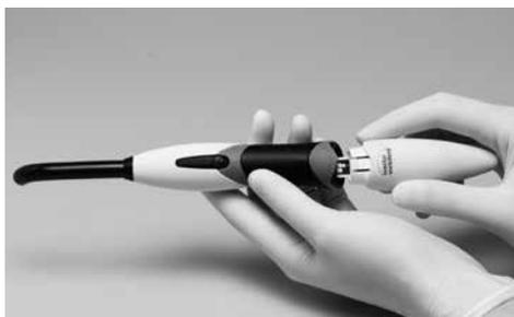
Gently place the handpiece in the corresponding rest in the charging base without using any force. If a hygiene sleeve is used, please remove it before you charge the battery. If possible, use the light always with a fully charged battery. This will prolong the service life. It is therefore recommended to place the handpiece into the charging base after each patient. If the battery is fully discharged, the charging time is 2 hours.
