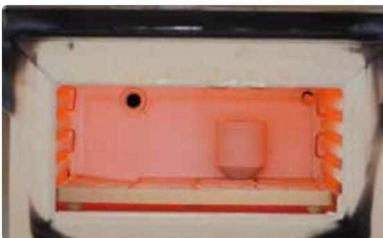
Place the investment ring in the predrying furnace with the opening facing down.
