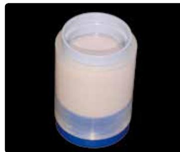
Fill the investment ring up to the marking and position the IPS Ring Gauge with a hinged movement. Press the ring gauge on the IPS Silicone Ring until it stops. Excess investment material escapes through the opening. Allow the investment ring to set without manipulating it.
