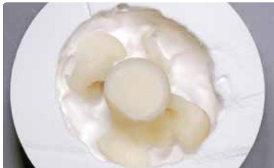
Rough divesting is carried out with polishing beads at 4 bar (58 psi) pressure until the objects become visible.
