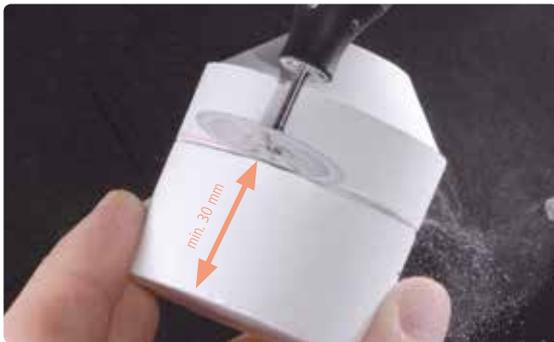
Separate the investment ring at a distance of at least 30 mm from the bottom surface using a separating disk...
