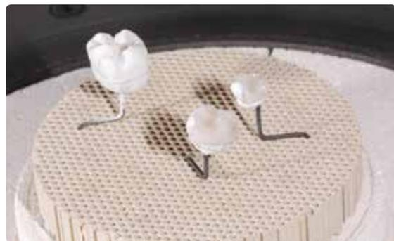
Conduct the Glaze firing on a honey-comb firing tray with the corresponding parameters.
