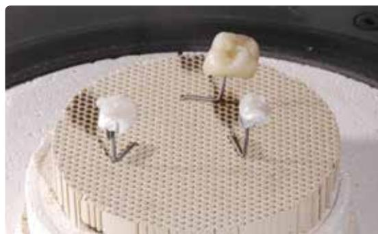
Conduct the Stain and Characterization firing on a honey-comb firing tray, an accessory of the ceramic furnace.
