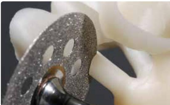
Separate the sprues with a thin diamond disk and provide permanent water cooling to the grinding area.
