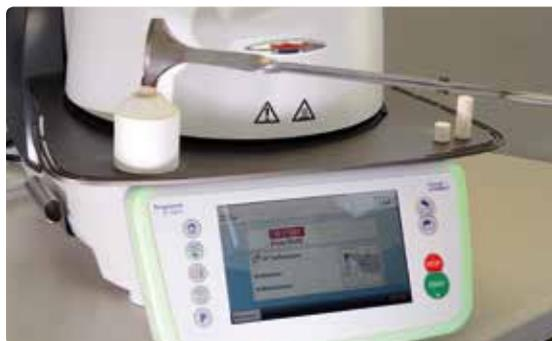
Place the **cold** IPS e.max Press Multi ingot into the **hot** investment ring with the rounded, blank side facing forward. The imprinted side faces upward to check the ingot shade.
