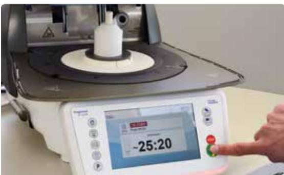
Place the completed **hot** investment ring in the centre of the **preheated** press furnace using the investment ring tongs. Press **START** to start the IPS e.max Press Multi program.
