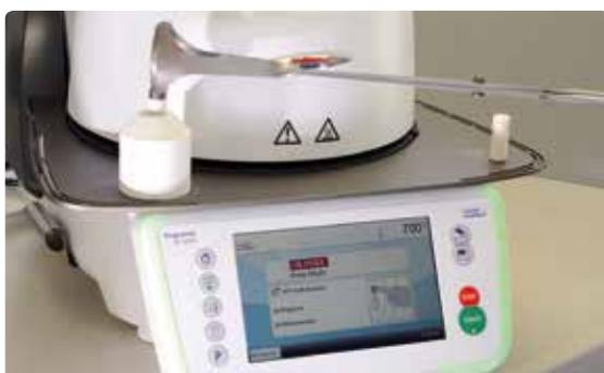
Place the **cold** IPS e.max Press Multi One-Way Plunger into the **hot** investment ring with the **chamfered side** facing forward.
