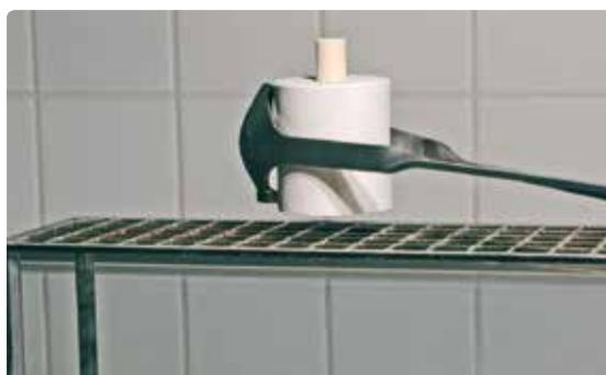
Once the press program is completed, place the hot investment ring on the cooling grid using the investment ring tongs and allow it to cool to room temperature.
