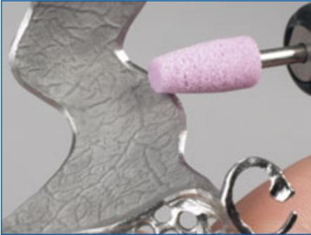
The non-fitting surface of the margins is also smoothed and tapered thinly with an abrasive stone.
