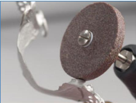
The residual sprues can be quickly and efficiently removed and smoothed with an abrasive disc.
