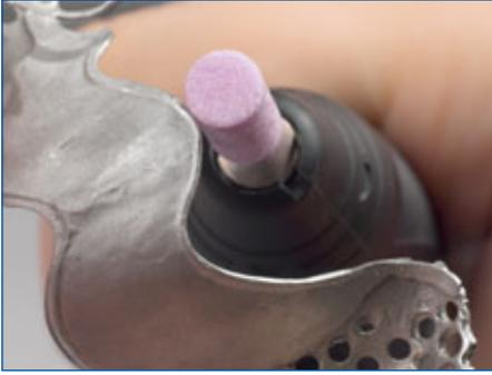
The margins of the transversal connector are prepared to a uniform contour with a coarse grit abrasive stone.
