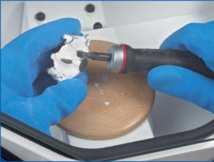
To avoid stresses in the CrCo framework, a pneumatic devesting chisel should be used for initial devesting.
