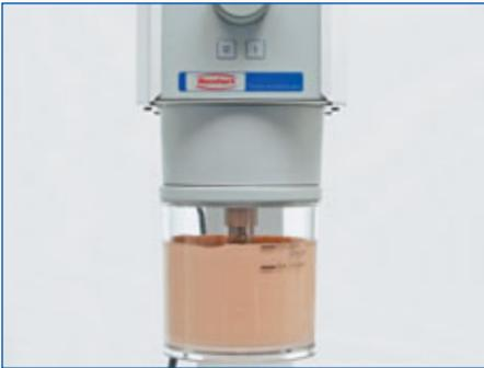
Use a Class IV dental stone for fabricating the working model and mix bubble-free in a vacuum mixer.
