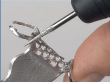
A tapered tungsten carbide cutter is used for preparing areas that are difficult to access.
