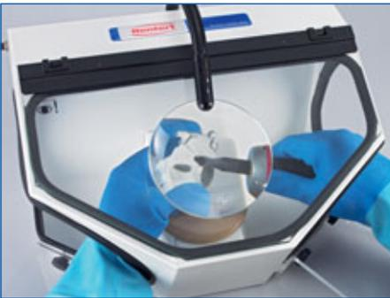
To avoid inhalation of hazardous quartz dust, castings should be devested in a dust extractor or in a suitable sandblasting unit.
