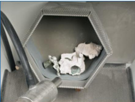
After initial devesting, the CrCo framework can be sandblasted in a fully automatic recycling sandblaster to save time ...
