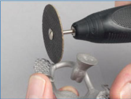
Separate the sprues approx. 1 mm/0.039 inch from the framework with a fibreglass reinforced cut-off wheel.
