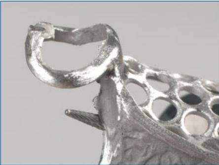
Any metal flash that is not part of the original pattern is also removed.
