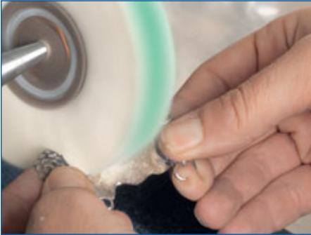
A pleated buff made from fine cotton and green high-lustre polishing paste are used to produce a high-lustre finish.
