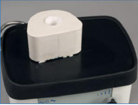
After the investment has completely set, the sleeve, base and crucible former are removed.
