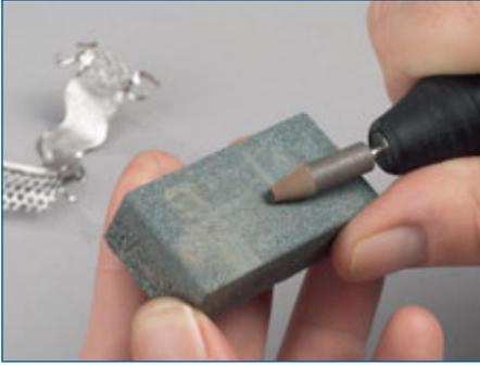
The polishers can be easily trimmed to the required shape with a dressing stone.
