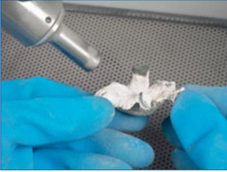
... or sandblasted manually, also in a recycling sandblaster.
