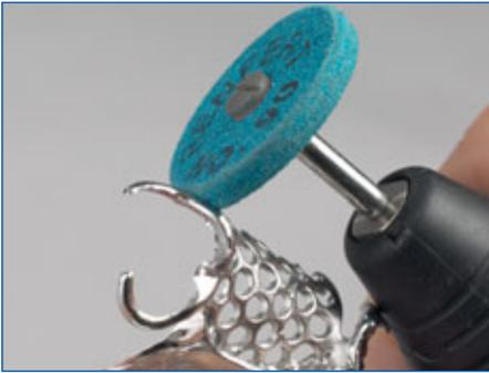
The polishing wheel is also used for prepolishing the non-fitting surfaces of the clasps.
