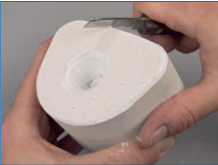
Sharp edges on the crucible and on the outer surface margins of the mould should be removed.
