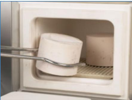
The mould can now be placed in the preheat furnace with the crucible opening facing downwards.
