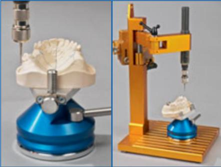
The model is securely clamped on a model table. A common path of insertion for the clasps is determined as follows using the surveying rod of the parallelometer.
