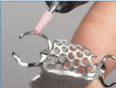
Flash is carefully removed from the edges of the clasps with a fine grit rotary instrument.
