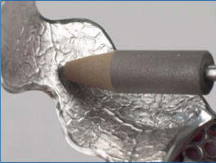
The stippled surface is also prepolished with a rubber polishing cylinder using light pressure. Ensure that the stippling is preserved when prepolishing.
