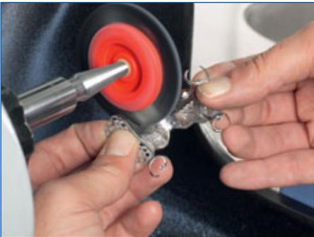
The CrCo framework is polished to a high lustre on the polishing motor with a special brush for CrCo and *Saphir* polishing paste.
