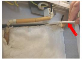
Fig. 41 – Installation of new muffle
