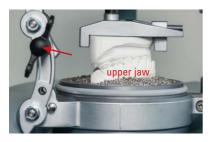
Hint: The construction dimensions of the Occluform-3 allow a bite elevation at average values. The elevation of 1 line at the supporting pin corresponds to approx. 1 mm bite elevation at the incisal point. If a construction bite is at disposal the models are articulated in the Occluform-3 using this construction bite.
