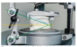
The construction of the Occluform-3 device is based on a Bonwill triangle with a side length of 11.5 cm (dashed triangle) and a Balkwill angle of 20°.
