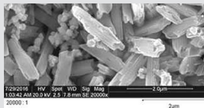
Conventional LS 2 Press ingot HT A2 Etched surface (Lithium Disilicate crystal - 1.8 µm)
