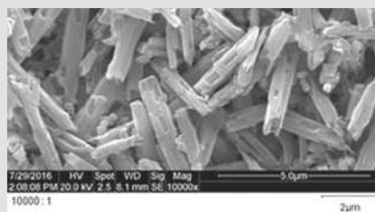
Conventional LS 2 ingot HT A2 Etched surface (Lithium Disilicate crystal - 4.2 µm)
