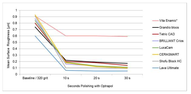
Fig. 17: Mean surface roughness of various composite-based CAD/CAM materials after polishing with OptraPol for 30 seconds. (Preclinic R&D Ivoclar Vivadent, Schaan, March 2018)
