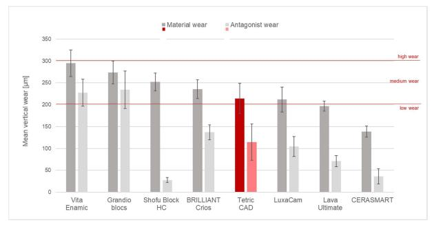
Fig. 10: Comparison of wear resistance (Willytec Method) of various composite block materials. R&D lvoclar Vivadent. Schaan, March 2018
