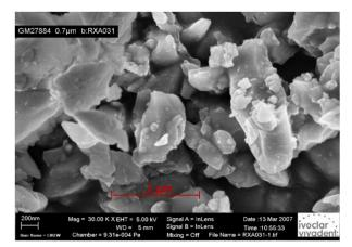
Fig. 3: SEM image of barium aluminium silicate glass filler with mean particle size of  $0.7 \mu m$
