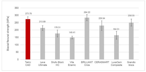
( $\emptyset$  = 12-16 mm, h = 1.2mm) of each of the composite blocks were prepared and loaded until breakage occurred. Specimens were stored in dry conditions until testing.
