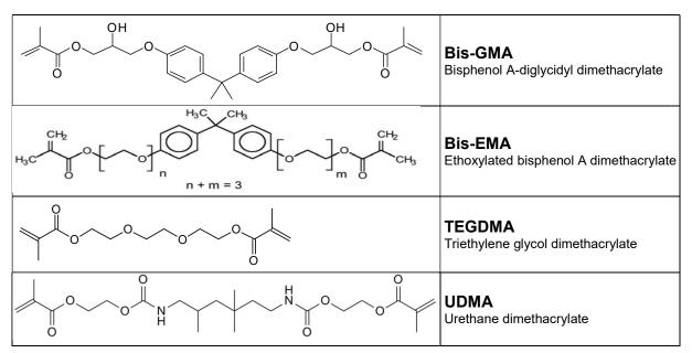
Tab. 1: Table illustrating the structural formulae of monomers used in Tetric CAD
