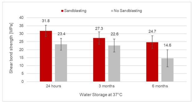
Fig. 12: Shear bond strength of Tetric CAD bonded with Adhese Universal and Variolink Esthetic DC with or without sandblasting. R&D Schaan, Ivoclar Vivadent 2018
