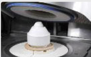
Place the **hot** and completed investment ring in the center of the **hot** press furnace using the IPS Investment Ring Tongs
