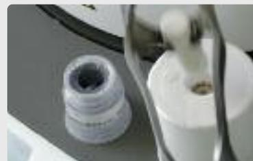
Then, place the powder-coated side of the IPS Alox Plunger into the **hot** investment ring.
