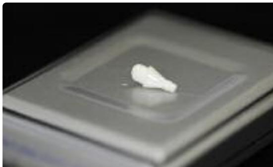
Weigh the abutment with the fired ZirLiner and record the weight.
