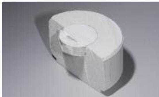
Separate the Investment Ring System 200 g including the One-Way Plunger at the marking using a separating disk. With the Investment Ring Systems 100 g and 200 g, separate the investment ring at the marking at the height of the Alox plunger.
