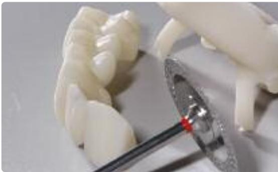
Use a fine separating disk and continuous water cooling to cut the sprues.
