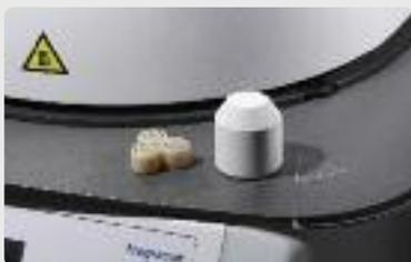
Provide a **cold** IPS Alox-Plunger and **cold** IPS e.max ZirPress ingots in the desired shade.
