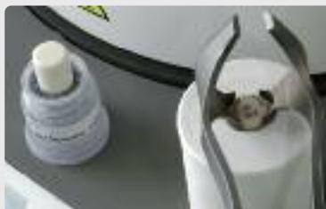
Place the **cold** IPS e.max ZirPress ingot into the **hot** investment ring, with shade imprint facing upward.
