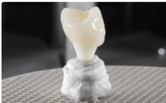
Conduct the Stain and Characterization firing on a honey-combed tray using the stipulated firing parameters.
