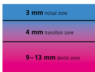
The dentin/incisal distribution in the unsintered IPS e.max ZirCAD Prime disc
