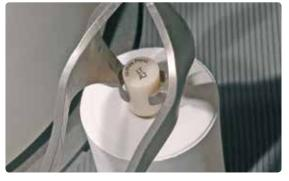
Place the  ${\bf cold}$  IPS e.max Press ingot into the  ${\bf hot}$  investment ring with the shade imprint facing upward.
