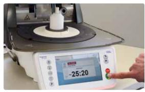
Place the completed **hot** investment ring in the centre of the **preheated** press furnace using the investment ring tongs. Press START to start the IPS e.max Press Multi program.
