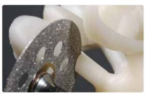
Separate the sprues with a thin diamond disk and provide permanent water cooling to the grinding area.
