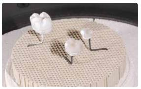
Conduct the Glaze firing on a honey-comb firing tray with the corresponding parameters.
