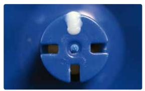
Seal the unused openings in the investment ring base with excessive amount of wax.
