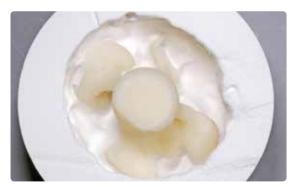
Rough divesting is carried out with polishing beads at 4 bar (58 psi) pressure until the objects become visible.
