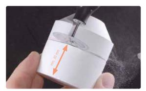
Separate the investment ring at a distance of at least 30 mm from the bottom surface using a separating disk...
