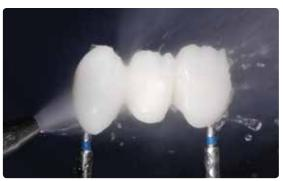
Blast the restoration with type 100 Al<sub>2</sub>O<sub>3</sub> at 1 bar (15 psi) pressure. Thoroughly clean the surface with a steam jet prior to the Wash firing and subsequently dry.
