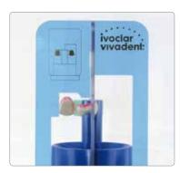
Attach the wax-up to the IPS Multi Investment Ring Base 200 g using the IPS Multi Wax Pattern. Check the correct positioning with the IPS Sprue Guide 200 g.
