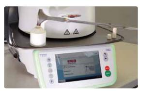
Place the **cold** IPS e.max Press Multi ingot into the **hot** investment ring with the rounded, blank side facing forward. The imprinted side faces upward to check the ingot shade.
