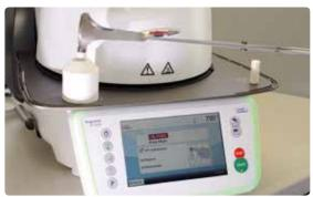
Place the  ${f cold}$  IPS e.max Press Multi One-Way Plunger into the  ${f hot}$  investment ring with the  ${f chamfered}$  side facing forward.
