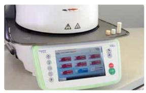
Provide a **cold** IPS Multi One-Way Plunger, a **cold** IPS Alox Plunger **and a cold** IPS e.max Press Multi ingot in the desired shade and select the press program for IPS e.max Press Multi.
