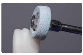
Smooth out the attachment points of the sprue using low speed and light pressure and
