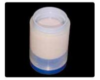
Fill the investment ring up to the marking and position the IPS Ring Gauge with a hinged movement. Press the ring gauge on the IPS Silicone Ring until it stops. Excess investment material escapes through the opening. Allow the investment ring to set without manipulating it.
