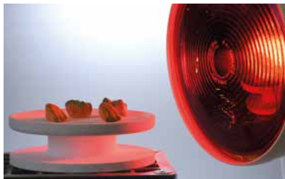
Drying of the infiltrated restorations under an infrared lamp
