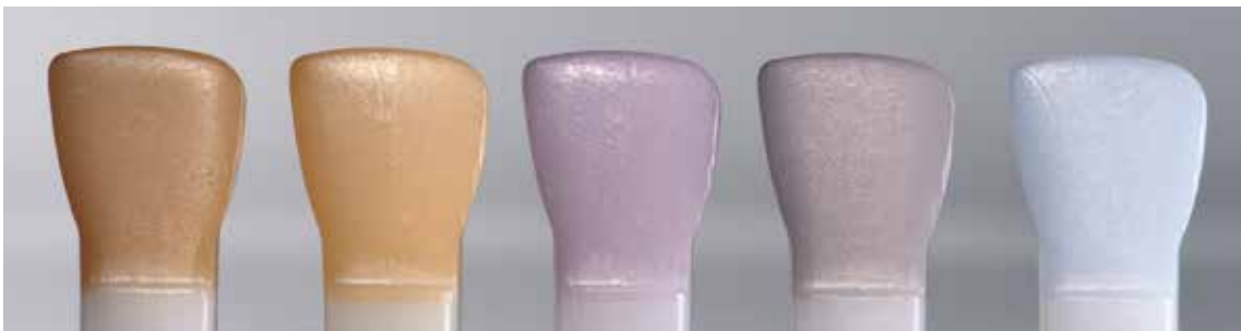
Shade tabs infiltrated with brown, orange, violet, grey and blue (from left to right).
