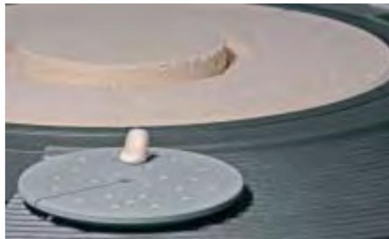
After the crystallization program, remove the firing tray from the furnace and allow the IPS e.max CAD restoration to cool to room temperature.
