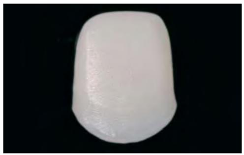
IPS e.max CAD framework after 35 minutes crystallization
