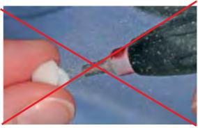
Do not remove residue with Al<sub>2</sub>O<sub>3</sub> or glass polishing beads.
