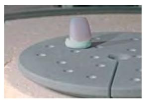
Place the firing tray in the furnace and start the crystallization program.
