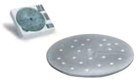
The large firing tray is used in the crystallization of IPS e.max CAD restorations. The firing pins contained in the refill must not be used for the crystallization of IPS e.max CAD or for firing IPS e.max Ceram. These firing pins are only used to support metal-ceramic restorations.
