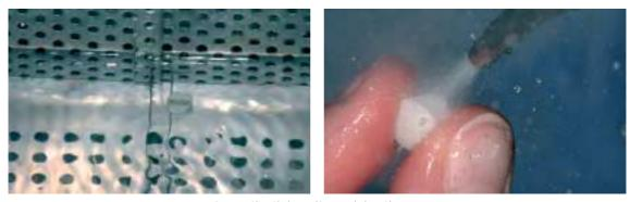
Remove residue with ultrasound in a water bath or with steam.
