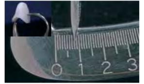
Make sure that the minimum thickness of the restoration is maintained during finishing.
