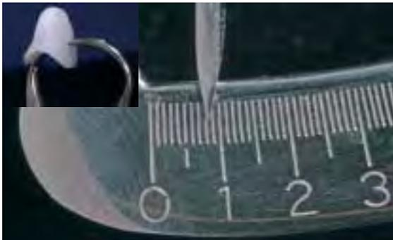
Make sure that the minimum thickness of the restoration is maintained during finishing.
