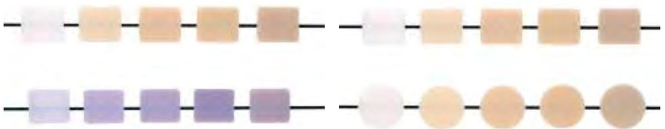
IPS e.max CAD before and after crystallization
