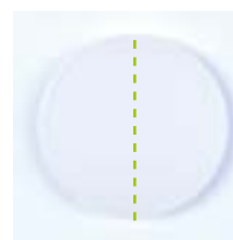
Variolink Esthetic Suntest (acc. to ISO 4049), left side exposed to light
