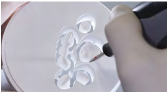
Fine tungsten carbide burs or diamond grinding instruments are recommended for separating the restorations. The holding bars have to be notched on one side before the restoration is completely separated.
