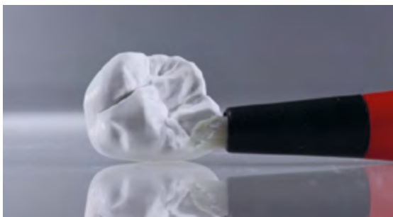
Thoroughly clean the zirconium oxide dust with a soft brush and then blast it with oil-free compressed air.
