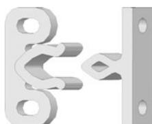
FIG. 274 SEPARATE LATCH: SOCKET LEFT, PLUG RIGHT
