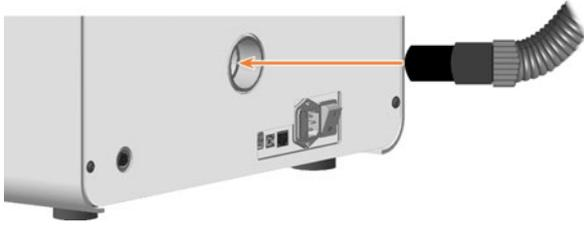
FIG. 65 INSERTING THE HOSE CONNECTION INTO THE OPENING FOR THE AIR EXTRACTION SYSTEM
