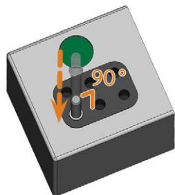
FIG. 44 INSERTING TOOLS INTO THE TOOL POSITIONS
