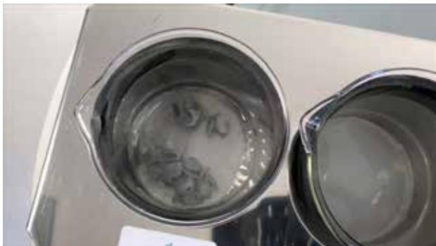
5. After cleanup, remove the 3D objects, rinse with water and light cure.
