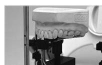
**i** Insert horizontal guide completely into the instrument carrier.
