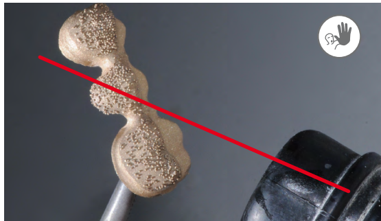
Carefully blast the framework with \text{Al}_2\text{O}_3 (80–100 \mu\text{m} ) and 2–3 bar (29–43.5 psi) pressure and tap off with an instrument.
