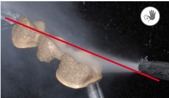
Carefully blast the framework with \text{Al}_2\text{O}_3 (80–100 \mu\text{m} ) and 2–3 bar (29–43.5 psi) pressure and tap off with an instrument.
