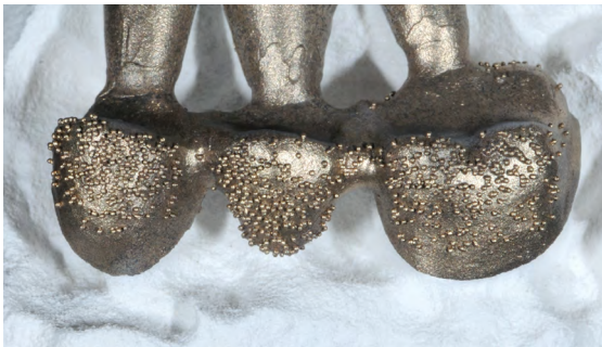
Carefully divest, blast/pickle and fit the framework on the model.
