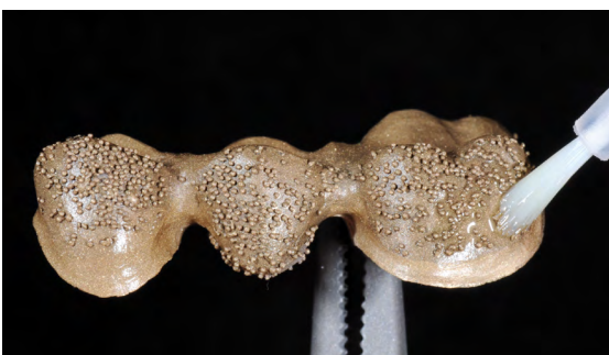
Immediately after the blasting procedure, tap off blasting medium residue, apply SR Link using a disposable brush and allow to react for 3 minutes.
