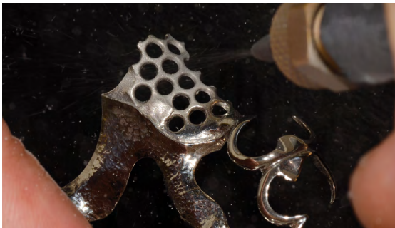
Carefully blast the retentions with \text{Al}_2\text{O}_3 , 80–100 microns at max. 3 bar (43.5 psi) pressure; then remove any residue by careful tapping with an instrument.
