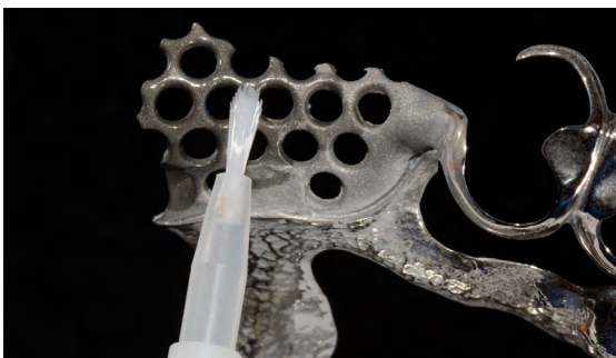
Apply SR Link immediately after the blasting procedure using a disposable brush and allow to react for 3 minutes.
