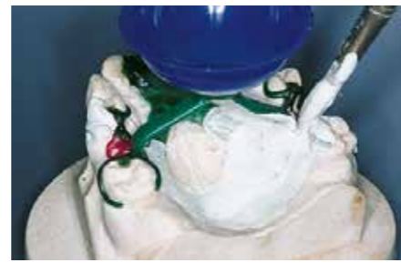
Very smooth casting surfaces with Wiropaint plus, model with molded base
