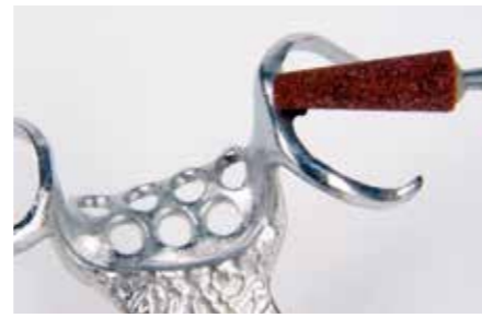
Finishing with corundum or fine grinding stones
