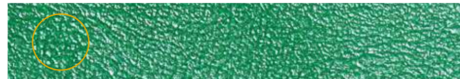
Stippled casting wax for waxing up the bases of upper partial dentures
