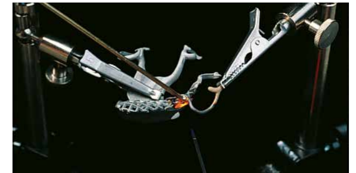
Soldering of a prefabricated gold clasp
